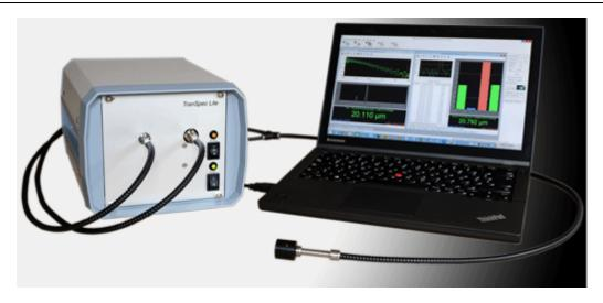
The **TranSpec Lite** film thickness gauges use the white-light interference phenomenon for non-contact and non-destructive layer determination of transparent single or double layers in the range of around 0.8 to 120 micrometers (depending on the model). The TranSpec Lite instruments are designed for manually performed, but even though high-precise measurements in the lab.
